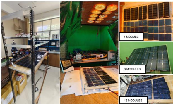
Figure 5 Photovoltaic Module Configurations used in Low-irradiance Testing
