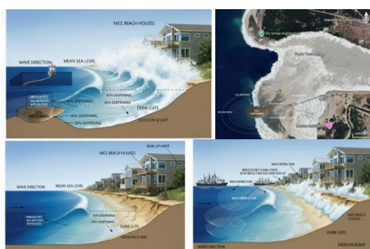
Figure 8a, 8b, 8c, 8d (from top left to down right) Impacts of Altered Bathymetry on Coastal Structures
