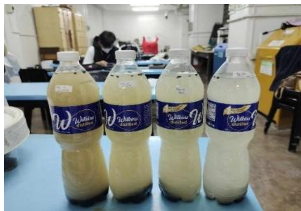
Figure 12 The photo taken from the representative replica of the 15, 20, 25 and 30g/L of AC over the Free Cyanide contaminated solution towards NaCN recovery in the Department of Mining Laboratory, Saint Louis University, Baguio City, Philippines.
