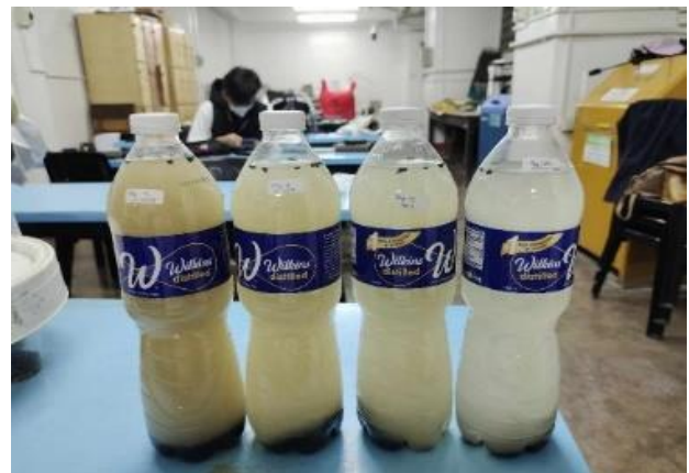
Figure 12 The photo taken from the representative replica of the 15, 20, 25 and 30g/L of AC over the Free Cyanide contaminated solution towards NaCN recovery in the Department of Mining Laboratory, Saint Louis University, Baguio City, Philippines.
